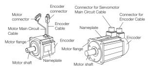
Note: The actual shape of the Servomotor depends on the series and model.
